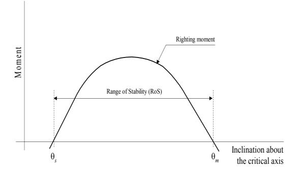
Figure 3-2 – Residual stability for self-elevating units
