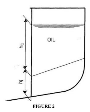
Where a double bottom does not exist, then  $h_c$  is to be taken at its maximum value considering any deadrise of the ship. Refer to figure 3.
