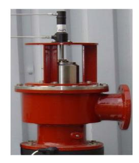
Figure 4.1 – Hydraulically controlled VOCON valve
