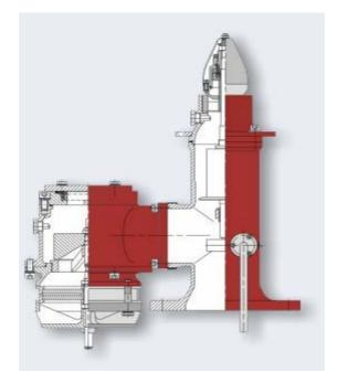
Figure 2.4 – A design and construction of a P/V valve<sup>2</sup>
