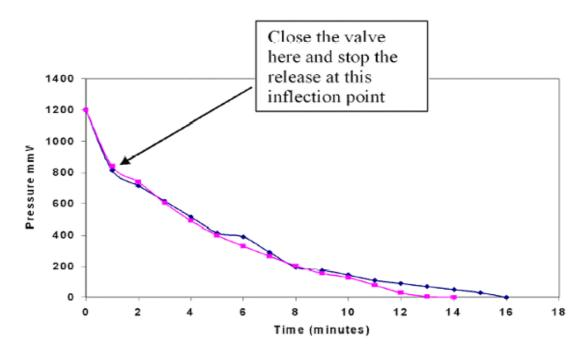
Figure 4.2 – A mast riser release
