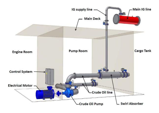
Automatic system operation is controlled by a dedicated pressure sensor installed in the main inert gas line, and is based on pre-set pressure levels determined by the crew. The CVOC system can also be operated manually as long as the cargo tank pressure is sufficient.
