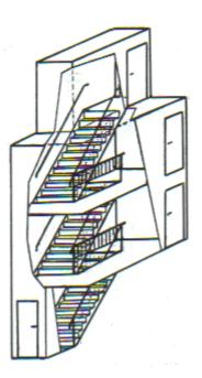
staircase well with going round entrances on each deck level, self-closing doors
