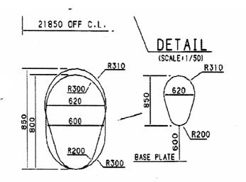
3 If a vertical opening is at a height of more than 600 mm steps and handgrips should be provided. In such arrangements it should be demonstrated that an injured person can be easily evacuated.
