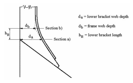
Figure 3 – Definition of the lower bracket web depth
