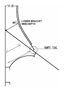
Figure 4 - Tripping brackets to be fitted in way of foremost hold
