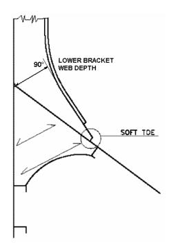
Figure 4 – Tripping brackets
