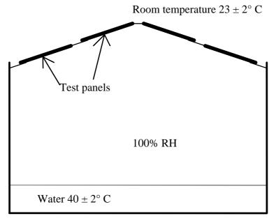
Figure 2 Condensation chamber
