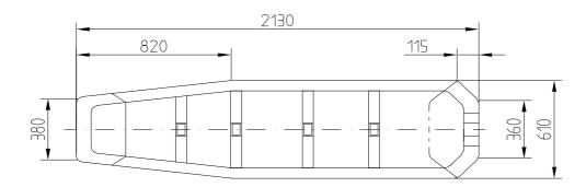
Figure 4 – Stretcher dimensions (mm)
