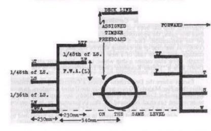
All lines are 25 mm thick. I.S. means Summer Timber Draught. F.W.A.(L) is Fresh Water Allowance equal to  $\frac{\Delta}{4T}$  mm where  $\Delta$  is the LS salt water displacement in metric tons and T is the metric tons per centimetre
