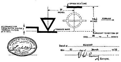
application, be placed above such tonnage mark at a distance of one forty-eighth of the moulded draught to that tonnage mark. This line must be 9 inches long and one inch wide measured from a one inch wide vertical line at the after end of, and perpendicular to, that tonnage
