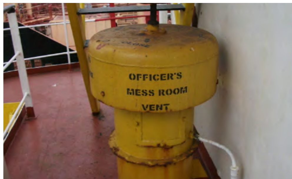
Fire damper that will not pass inspection
