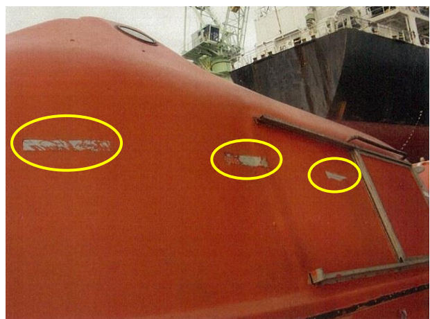
Retro-reflective tape deteriorated.
