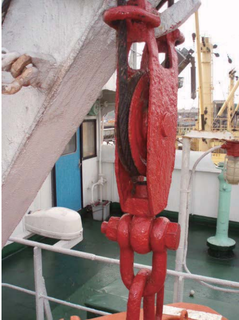
Wastage of boat fall block
