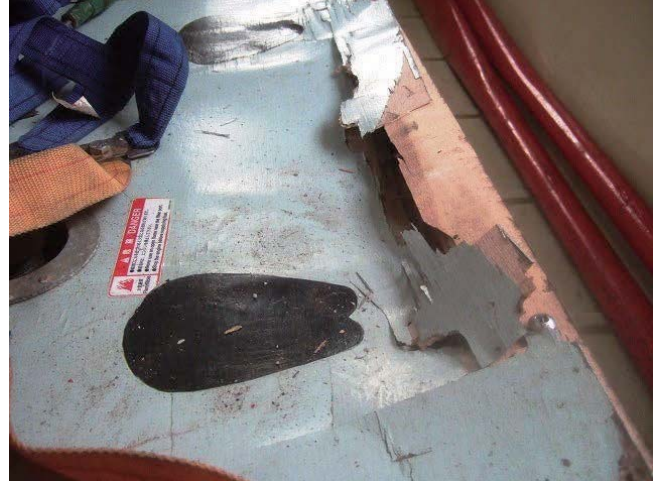
Damaged lifeboat seat
