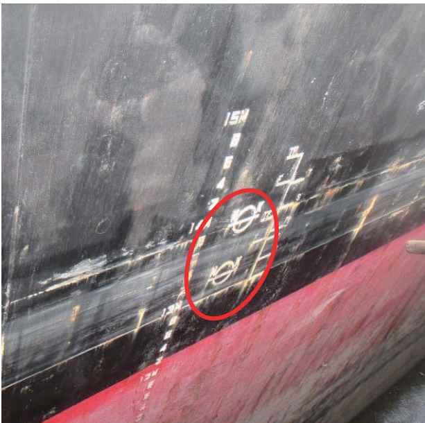
Double marks (Not acceptable)
